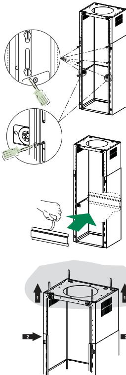
Before final locking of the screws it is possible to make small adjustments to the frame, making sure that the screws do not come out of the adjustment slot.
