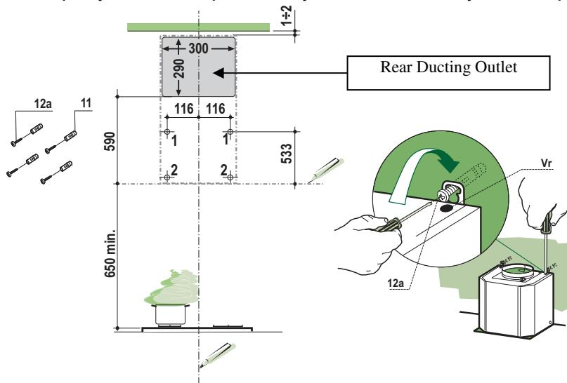
If the hood is fitted in the recirculation version, bear in mind that there must be a minimum distance of at least 8-10 Cm left between the top of the hood and the surface above it (ceiling or shelf).
